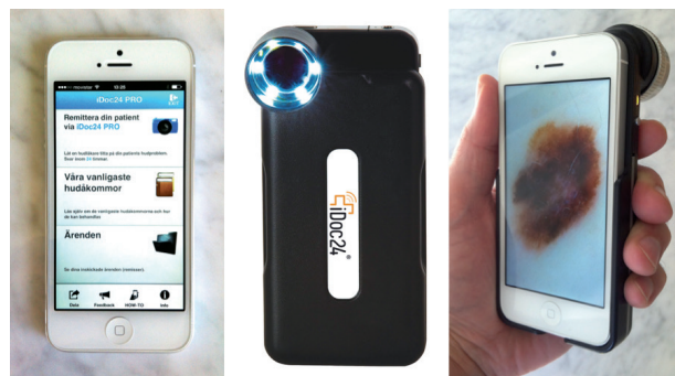
Fig. 2. Images of the first smartphone app for TDS (iDoc24® PRO), which used a digital dermoscope (Handyscope®, Fotofinder®) coupled with an iPhone® 4.
