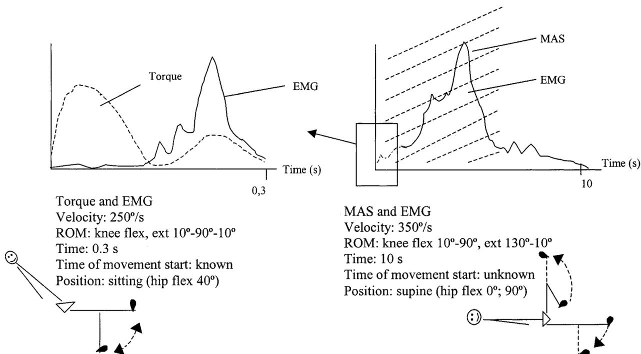
Fig. 1. Description of time course and temporal relationship between recordings. The hatched area in the upper panel indicates the approximate time interval when the investigator makes the Modified Ashworth Scale (MAS) estimate.
