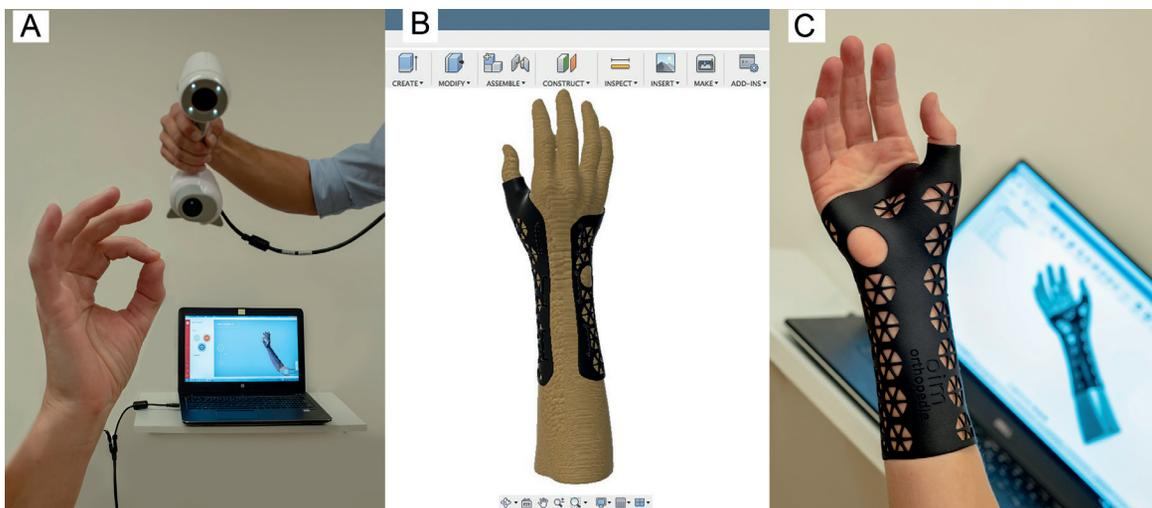
**Fig. 2.** Production process of the 3-dimensional (3D)-printed orthosis. (A) Scanning the hand and forearm, (B) designing the orthosis based on the digital model of the hand, and (C) the 3D-printed orthosis.
