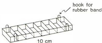
Fig. 1. Feeding capsule for larvae of the human head louse, divided into different compartments. The capsule was fixed to the underarm with two rubber bands.
