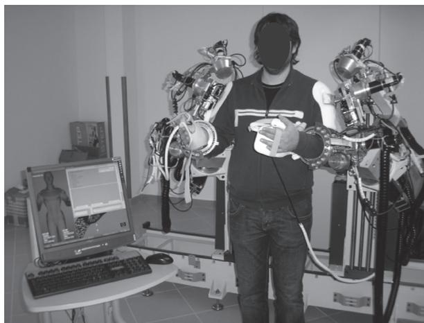
Fig. 1. The robot ARAMIS (Automatic Recovery Arm Motility Integrated System).
