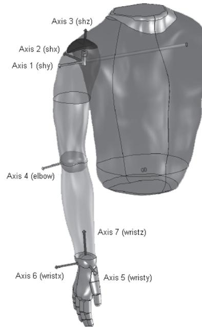
Fig. 2. Links and joints of a robotic manipulator.
