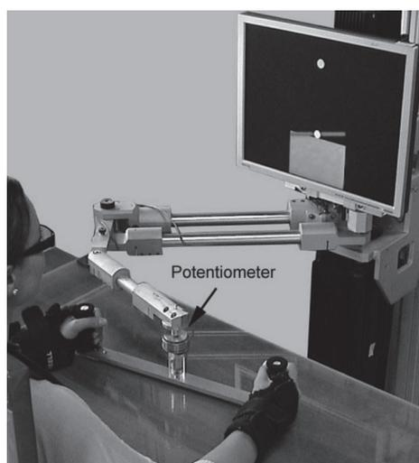
Fig. 1. The haptic robot Braccio di Ferro, modified by mounting a horizontal bar for bimanual co-ordination. The bar is free to rotate around a vertical hinge. The rotation angle is measured by a potentiometer. The computer screen displays the target and the position/orientation of the bar. The task is to reach the target with an approximately horizontal bar ( $\pm 4^\circ$ ). Note the wrist holders, used in skate-boarding.
