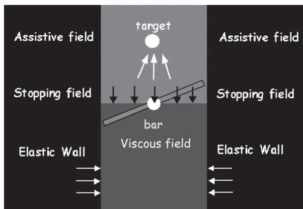
Fig. 2. Combination of force fields implemented by the robot for the designed experimental protocol: (i) an assistive force field directed from the hand to the target; (ii) a stopping field, activated when the orientation error exceeds the threshold ( $\pm 4^\circ$ ); (iii) an elastic wall, for avoiding large lateral deviations from the nominal straight trajectory; and (iv) a viscous field for damping oscillations.
