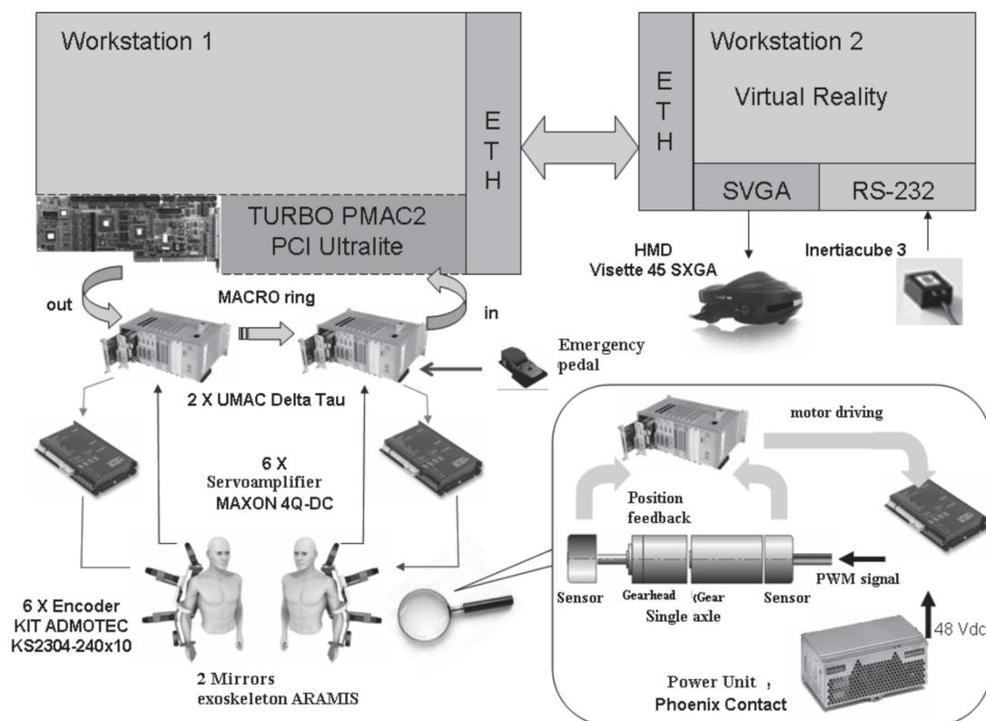
Fig. 2. Hardware architecture of the Automatic Recovery Arm Motility Integrated System (ARAMIS).
