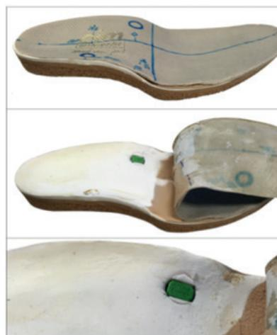
Fig. 1. Custom-made inlay with built-in sensor.
