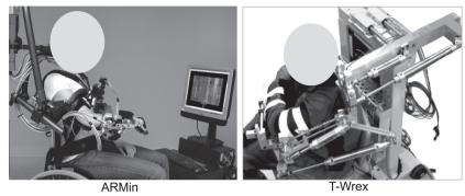
Fig. 3. Examples of exoskeletons.
