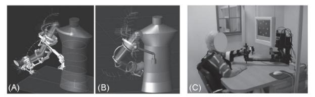
Fig. 1. An exoskeleton representation with related potential degree of freedom (A, B) and an example of operational type machine with training feedback on the monitor (C).
