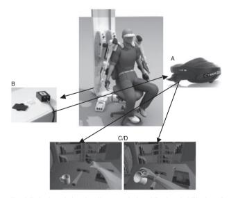
*Fig. 1.* Robotic and virtual reality setup designed for the rehabilitation of the upper limb after stroke. (A) Head-mounted display Visette 45 SXGA (Cybermind B.V., Maastricht, the Netherlands). (B) 3DOF visual tracking system. (C and D) Examples of interacting virtual environment as seen by the patient undergoing treatment.
