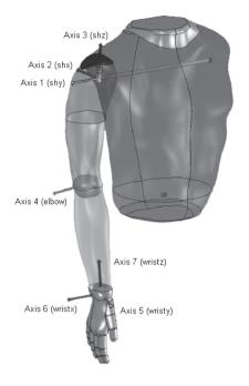
Fig. 2. Links and joints of a robotic manipulator.
