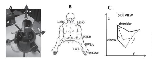
*Fig. 1.* (A) The 3 degrees of freedom (3DOF) robot. (B) Rear view of marker locations on the trunk and upper limbs. (C) Elbow and shoulder angles in one subject; the arrow indicates the movement direction along the dashed line.
