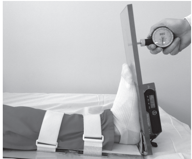
Fig. 1. Ankle range of motion measure device using standardized torque (13).
