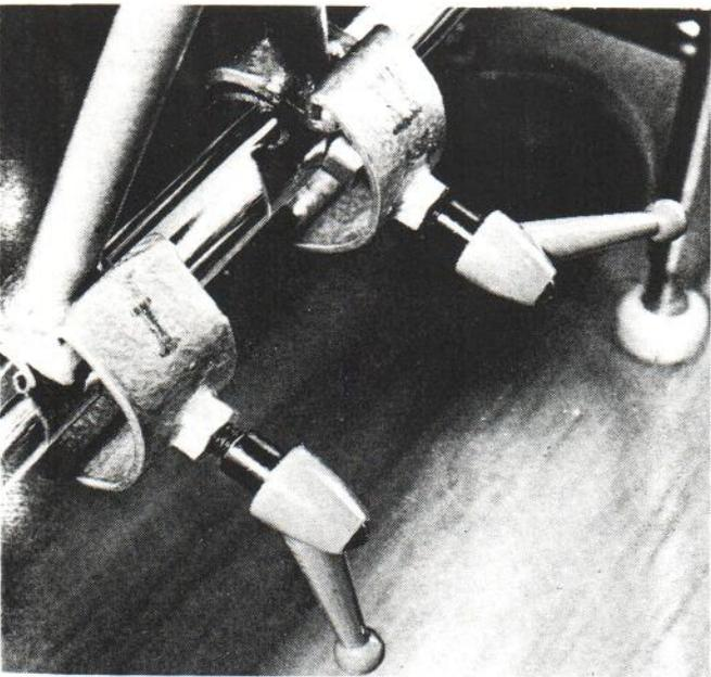
Fig. 2. Attachment to the bed frame with screws which enable the crutch to be lowered under the bed easily and rapidly.
